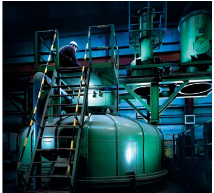
Materials are processed in one of Firth Rixson's two vacuum furnaces, such as this unit in Derbyshire, UK, designed to handle heats up to 12,000lb.
